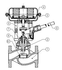
VPA26S- with pneumatic actuator and manual operation
